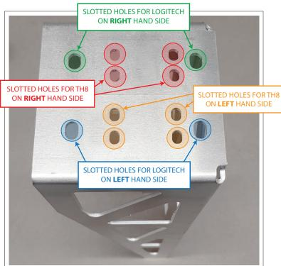
Mount your Logitech shifter to the alloy bracket using two M6x20mm hex bolts, two M6 washers and the slotted holes indicated (blue if using the shifter on the right hand side, or the green holes if using the shifter on the left hand side).
